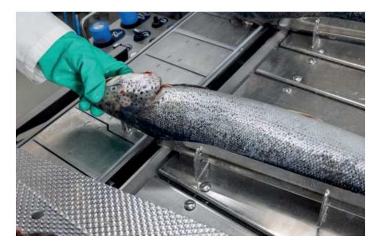
The Salmon Deheader MS 3028 provides consistent and efficient automated deheading to salmon processors. Built on the industry-leading legacy of the Curio Deheader, the MS 3028 offers next level accuracy to increase yields while reducing dependency on manual labor.
