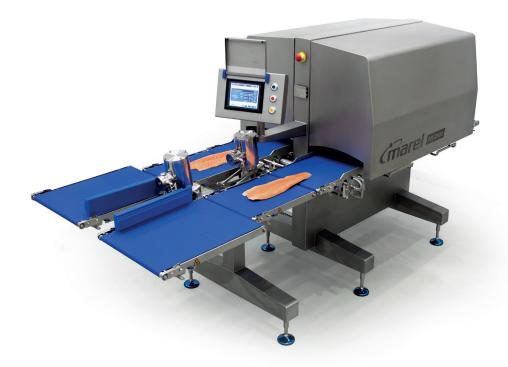
The QC Scanner MS 2920 monitors the quality of your salmon fillets in real time with detailed scans of the meat side for trimming, quality, color, and estimated weight calculation.
