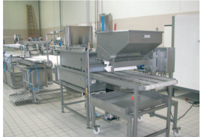
Marel fillet washer integrated into a filleting line.
